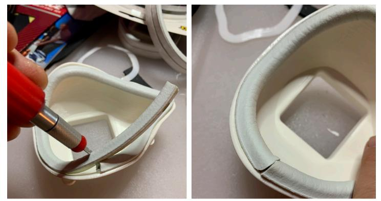
Use an exacto knife to cut the face seal so both ends abut to form as much of a seal as possible. Glue will fill the rest (see below).
