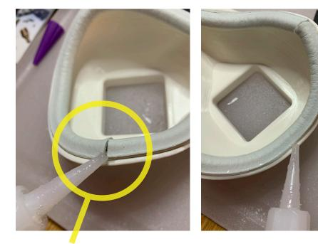
Glue at the junction point at both ends of the face seal first. This THE MOST CRITICAL GLUE POINT as there is a natural break in the seal. Glue this very well, very carefully. Put glue inside the seal, around it, etc. Squish out any air bubbles.
