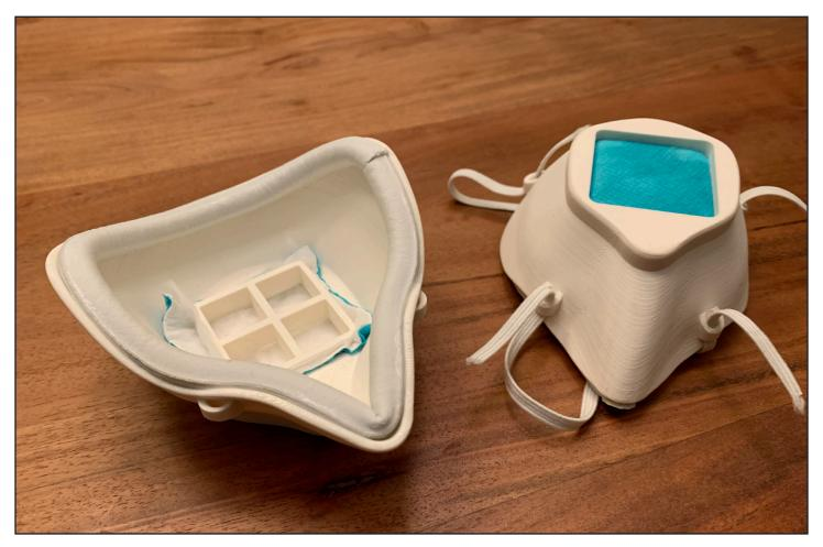
Two finished masks (although I haven't put in the INNER FACE SEAL GASKET yet on these two) with small squares of N95 material "sandwiched" in-between the main mask part and the window part. NOTE: This can create a very tight fitting...whcih may require you to sand the outside edges of the window part (all four sides) to get it to go in easier (to sandwich). Just depends on your printer, material, etc.
